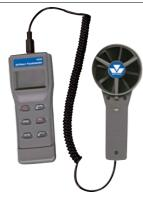
Reads Humidity, Air Temp., Dew Point, Wet Bulb, Air Velocity, Air Volume & BTU. The sensor is built into the remote fan and is protected by a rotating cap.
