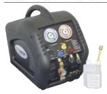
This unit offers all the same functions and features as the reliable 69000 recovery machine. In addition, Mastercool has strategically placed an oil separation module inside the unit that will dispense used oil effortlessly. Together with its filter dryer and sight glass this unit allows for the technician to actually clean the used refrigerant and potentially re-use.
