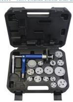
Pneumatic brake caliper piston compressor kit constructed of light weight durable anodized aluminum. Right or left hand wind-back operation for rear brake caliper pistons. Pneumatic single piston press shaft operation allows one technician to perform the brake job.
