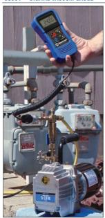
As a professional technician the assurance of a deep vacuum on a system is imperative. The main problem with many small handheld units is their inaccuracy and durability. Although the thermocouple sensor has been proven to be much more accurate and durable than the thermister type, the problem has been the inconvenience of a cumbersome tableton unit.
